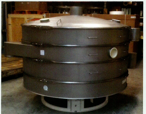
AMKCO 84" Separator was designed for larger flow rates. Increase screen area gives higher screening capacity.
