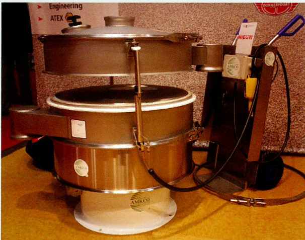
AMKCO pneumatic powered lift system is designed for quick and easy screen change with the use of two compact air cylinders.
